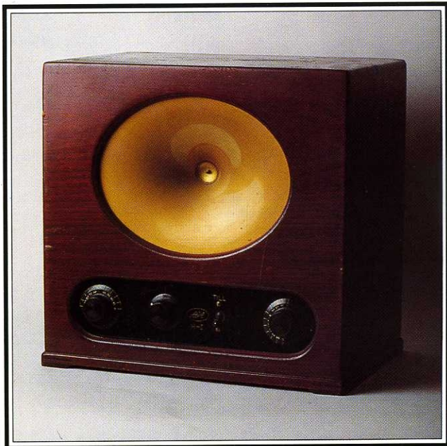
Reputed to be the first mains set with an integral loudspeaker, the 'H - I' was made for operation from 200V DC in around 1926 - 27 by the Swedish Aga Company, now more famous for its solid-fuel cooking stoves
