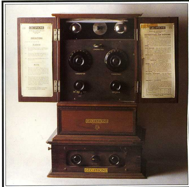
The Gecophone Model BC2001 2-valve set (1922) sitting on its matching 2-stage LF amplifier Model BC2580. The mahogany case was designed to resemble a 'smoker's cabinet', and the set became known by that name
