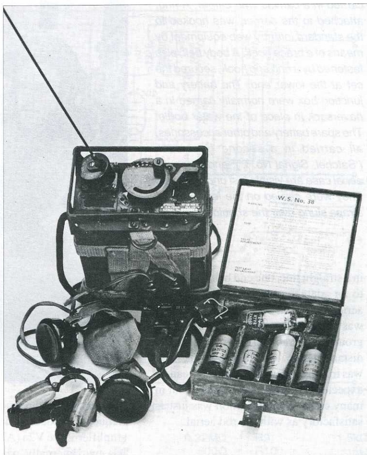
Wireless Set No.38 MkII* showing front panel of the set. On the left the aerial base in which a thin 4ft 'F' type aerial rod has been placed. In the centre the tuning dial with lock nut; and on the right the combined 'off-send-receive' switch. Lying in front of the set is 'Junction Box No. 2'. The dry battery, 'phones and throat-microphone are connected to the set by plugs and leads to the junction box. In the right of the picture a metal spare-valve box. Remarkable is an abridged fault location procedure, attached to the inside of the lid
